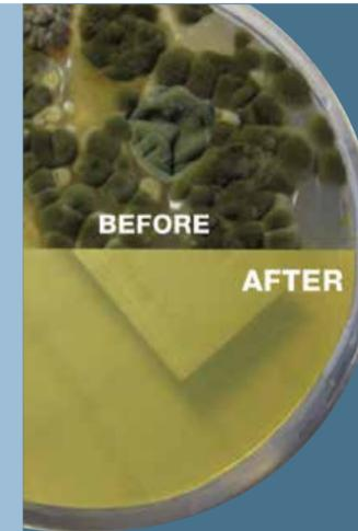
HVAC coil Petri dish samples demonstrate high concentrations of microorganisms.
