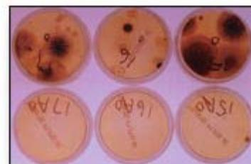
*The Petri dish samples (top row), taken from an HVAC coil, demonstrate high concentrations of bacteria, mold and yeast. After exposure to a UVC Emitter (bottom row), these microbes are almost completely eliminated.*
