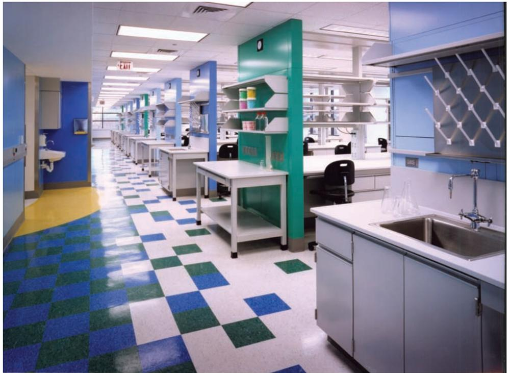
**Laboratories are designed on a generic footprint and incorporate a movable laboratory wall system and a flexible casework system to give users the capability of reconfiguration as technology or staff changes. Photo: Aker/Zvonkovic Photography**
