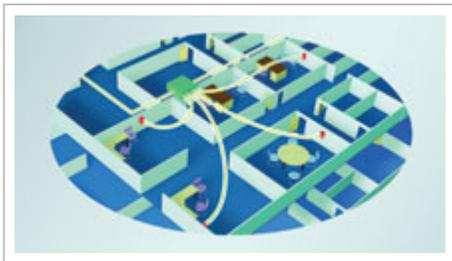
This illustration demonstrates a ventilation efficiency monitoring system installed in an office environment. Red squares represent wall-mounted sensors, yellow lines represent the cable through which air samples are routed and the green box is an air data router that sequences the air samples and routes them to a centralized sensor suite.
