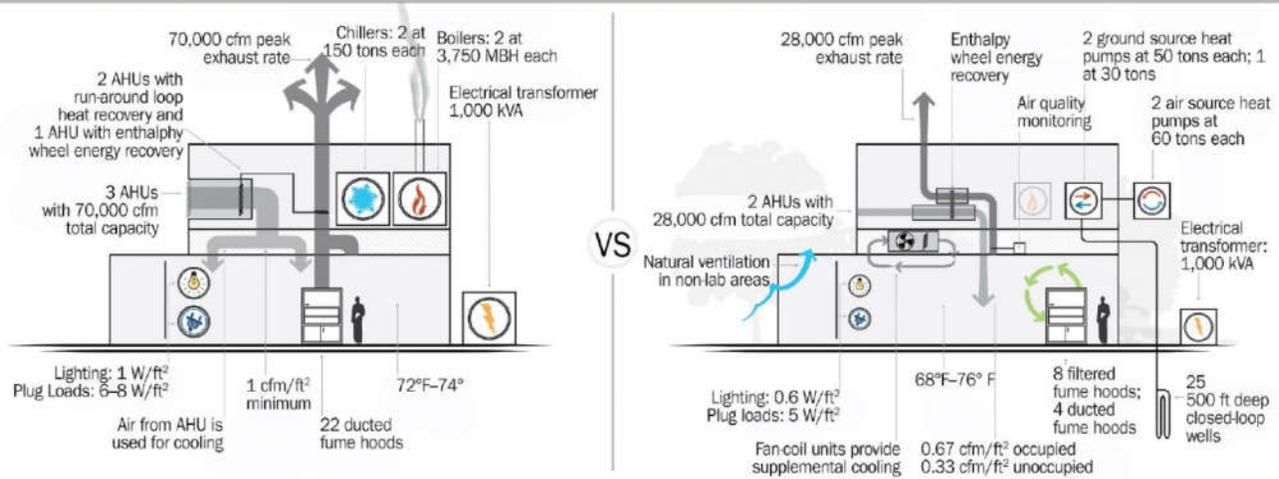
For every premium paid for a sustainable technology, a savings was found somewhere else, the result of an open and fruitful collaboration between the architect and engineer (*Figure 1*) illustrates these and other nuanced changes made between the two designs.
