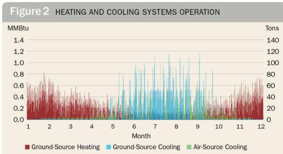
The amount of heat energy extracted from or rejected to a thermal mass is a product of the thermal mass and the change in temperature. To reduce the amount of thermal mass (well-field size), the seasonal temperature swing in the ground of 45°F to 60°F was expanded. Therefore, after a summer of rejecting heat from the building, the ground temperature may approach 90°F maximum, while after a winter of extracting heat from the ground, the ground temperature may approach 30°F minimum.
